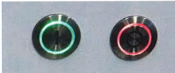
Figure 4.6: Power-off button in red on the right
